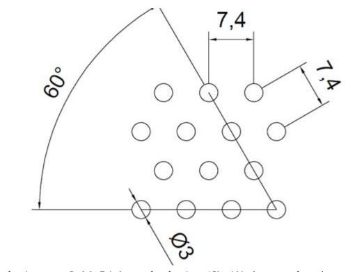
Perforation pattern Rv 3.0 - 7.4; degree of perforation = 15% within the area perforated.
