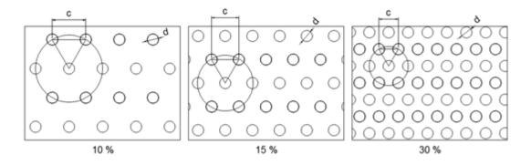
10 % perforation, hole size d = 4 mm, centres c = 12 mm
