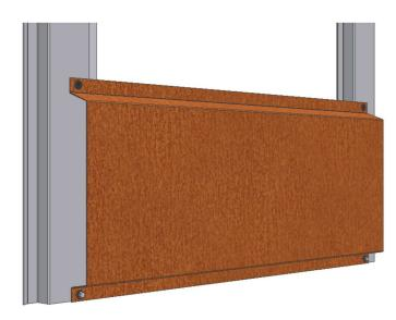
1. Add EPDM grommets to the upper and lower edges of the lamella. Add fasteners to the lower edge of the lamella, the joint should be at the center of the stud.
