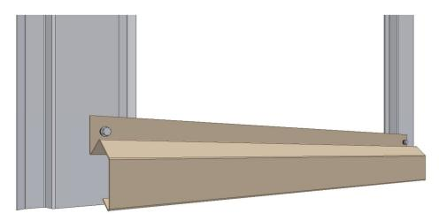
1. Add fasteners to the upper edge of the starting fillet CA1SF3, the joint should be at the center of the stud.
