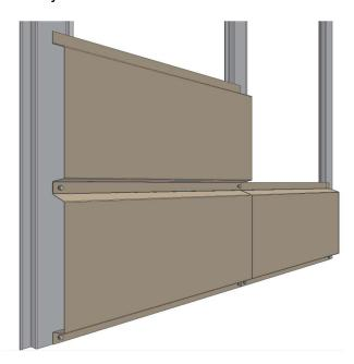
3. Install next row of lamellas by placing them on top of the bottom lamella and fastening through both flanges.
