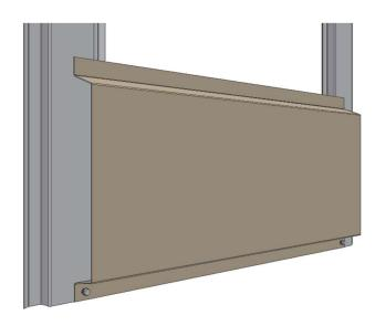
1. Add fasteners to the lower edge of the lamella, the joint should be at the center of the stud.
