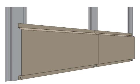
2. Continue installing the first row. Leave a 2-3 mm vertical gap between them for thermal expansion.
