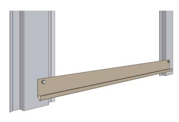
1. Add fasteners to the upper edge of the starting fillet CA1SF5, the joint should be at the center of the stud.
