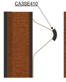
4. At the overlapping add separating strip CA3SE410 and fasteners to the lowest wave bottom
