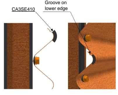
4. At the overlapping add separating strip CA3SE410 and fasteners to the lowest wave bottom
