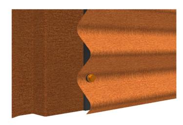
2. Add fasteners to the lowest wave bottom
