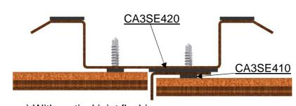
a) With vertical joint flashing
