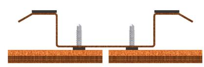
b) Without vertical joint flashing
