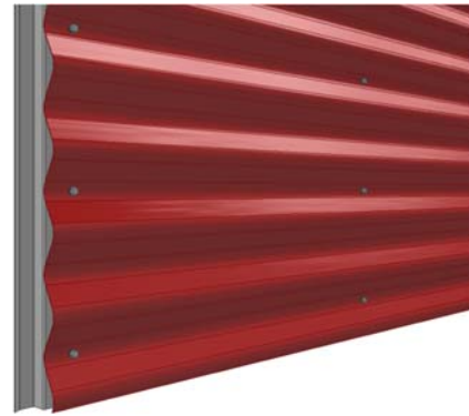
2. Add fasteners to the bottom of every second wave
