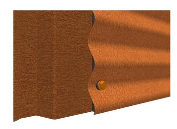
2. Add fasteners to the lowest wave bottom
