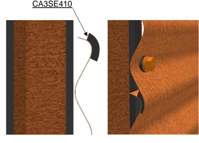
4. At the overlapping add separating strip CA3SE410 and fasteners to the lowest wave bottom
