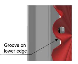
3. At the overlapping, add fasteners to the lowest wave bottom
