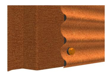
2. Add fasteners to the lowest wave bottom
