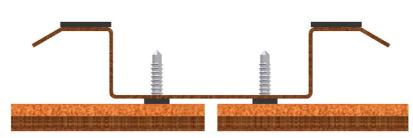
b) Without vertical joint flashing
