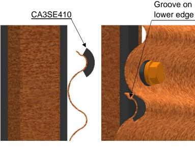
4. At the overlapping add separating strip CA3SE410 and fasteners to the lowest wave bottom
