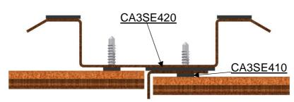
a) With vertical joint flashing
