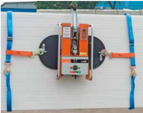
Pic. 3. Self-clamping tools.
