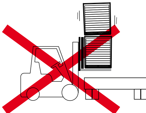
Fig.7 Packages should be unloaded one by one. Lifting two packages at once may damage a first panel in the first package.
