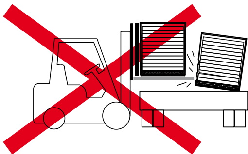
Fig.6 Too long forks may damage the second row of packages.
